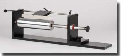
The VersaMount 24 can accommodate a wide range of printing cylinder widths with repeat lengths up to 24". The printing cylinder is securely positioned between two tapered centers, accepting a wide range of printing cylinder inside diameters without the need for adapters. A pivoting straight edge aids in drawing guide lines and cutting mounting tape.
